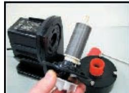
impeller the whole magnetic anchor out of its housing. At all times, avoid sideways pressure on the ceramic axle (only pull in the line of the axle). If you wish, you can now clean the inside of the magnetic motor.
